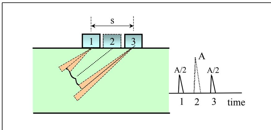
**Figure 4. Principle of dB drop technique**
