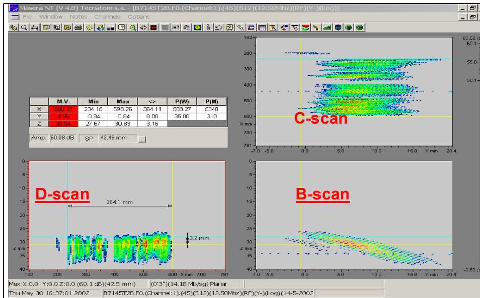
Figure 5. Example of intergranular stress corrosion crack sizing
