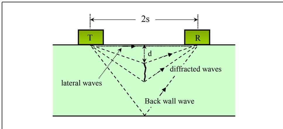
**Figure 3. Principle of TOFD technique**
