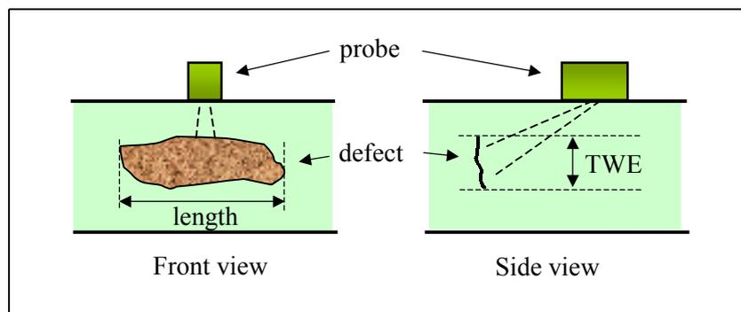
**Figure 1. Characterisation of a defect**
