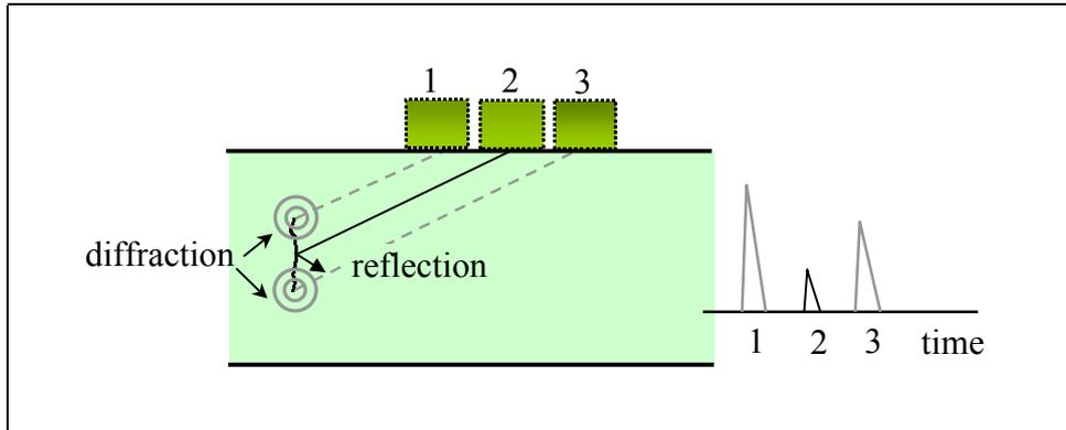
**Figure 2. Principle of backward scattering method**
