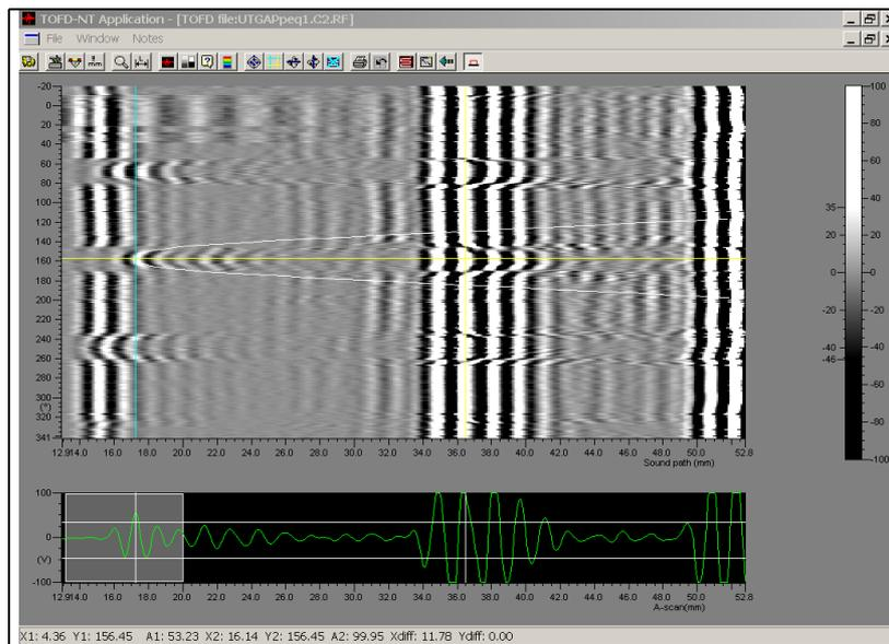
**Figure 7. TOFD technique sizing an artificial planar reflector**
