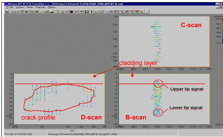
Figure 6. Image of a fatigue crack by backward diffraction method
