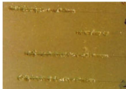
Figure 5: Scratches on sample D (CrN)
