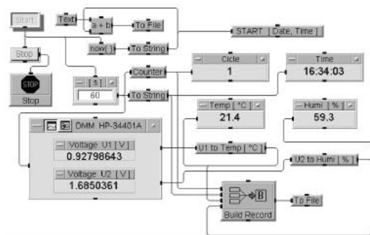
Figure 3: A basic part of the application program, written in the graphical programming language, for measurements at characteristic of the ultrasonic measuring chamber.
