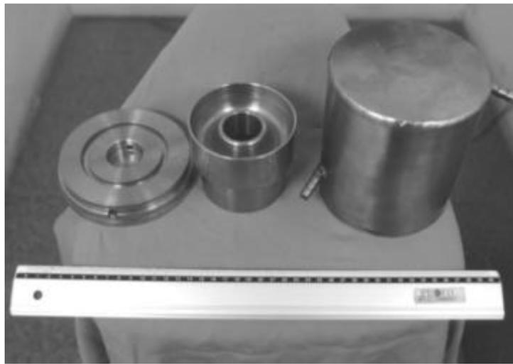
Figure 2: Dismantled ultrasonic measuring chamber for hydration kinetics measurements by ultrasonic shear waves.
