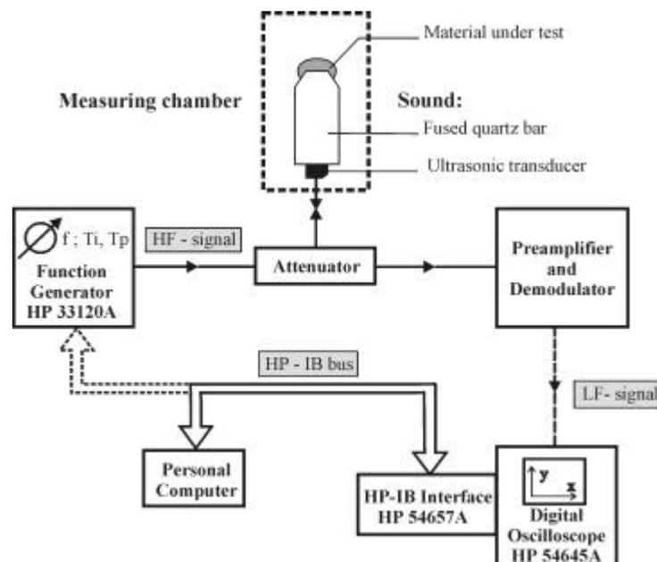
Figure 1: Block Scheme of the laboratory experimental setup for the cement mortar thickening time measurements by defining the amplitudes of the first two reflected HF ultrasonic shear waves.
