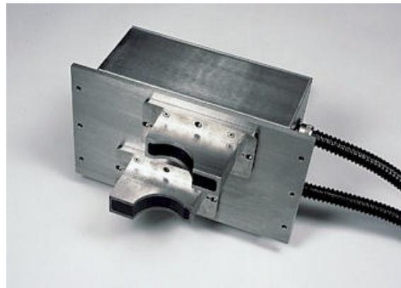
**Fig. 15: Phased Array Probe for tube inspection**
