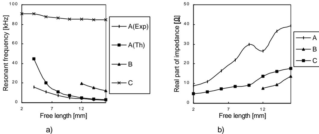
Figure 3 - a) Resonant frequency versus free length and b) real part of impedance versus free length for the three resonance modes.
