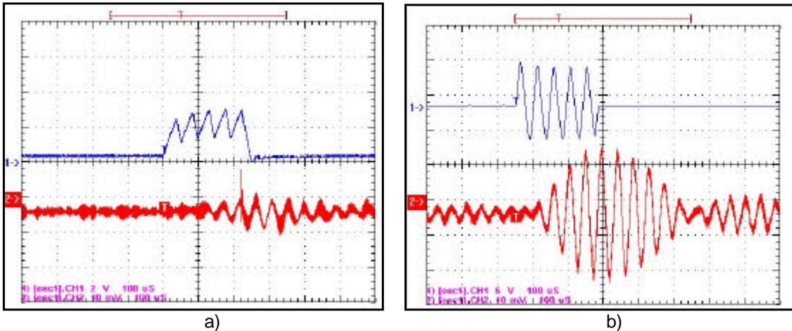
Figure 4 – Impedance matching influence: a) without matching b) with matching. Top signals are at the emitter and bottom signals are at the receiver.
