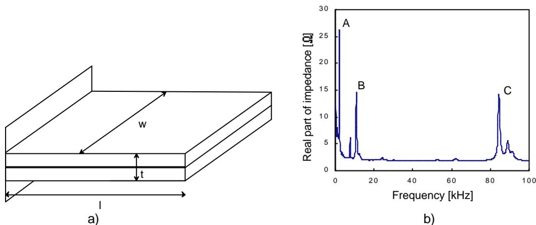
Figure 2 - a) Structure of a cantilevered bimorph actuator and b) frequency response of the cantilever with  $l=16$ mm.
