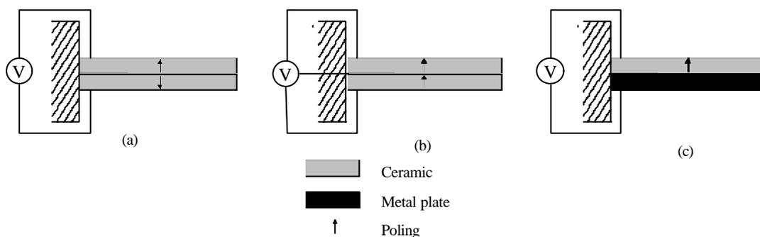
Figure 1 – Schematically configuration of bimorphs and unimorphs.
