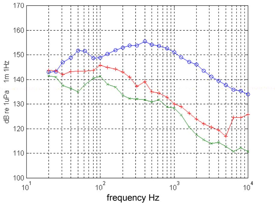
Figure 3.- Acoustic signature of the ships Cornide de Saavedra (blue); Vizconde de Eza with keel down (green); Vizconde de Eza, keel retracted (red). Speed 4 knots.
