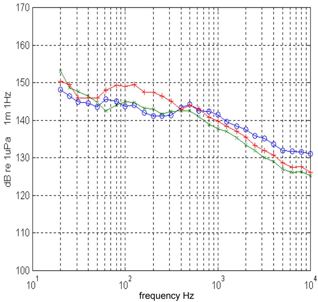
Figure 4.- Acoustic signature of the ships Cornide de Saavedra (blue); Vizconde de Eza with keel down (green); Vizconde de Eza, keel retracted (red). Speed 10 knots.
