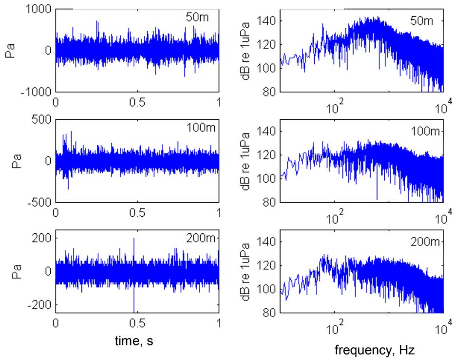
Figure 2.- Temporal sample, and frequency spectrum, in dB re. 1  $\mu$ Pa, of the noise radiated by the ship Cornide de Saavedra, 4 knots, port side.
