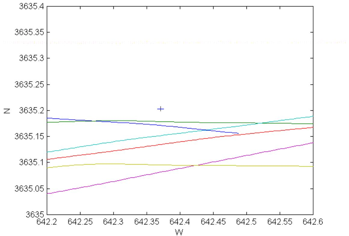
Figure 1.- Trajectories of the ship Cornide de Saavedra at 10 knots. Dark blue, port, 50 m. Dark green, starboard, 50 m. Red, port 100 m. Light blue, starboard, 100 m. Magenta, port, 200 m. Light green, starboard, 200 m.
