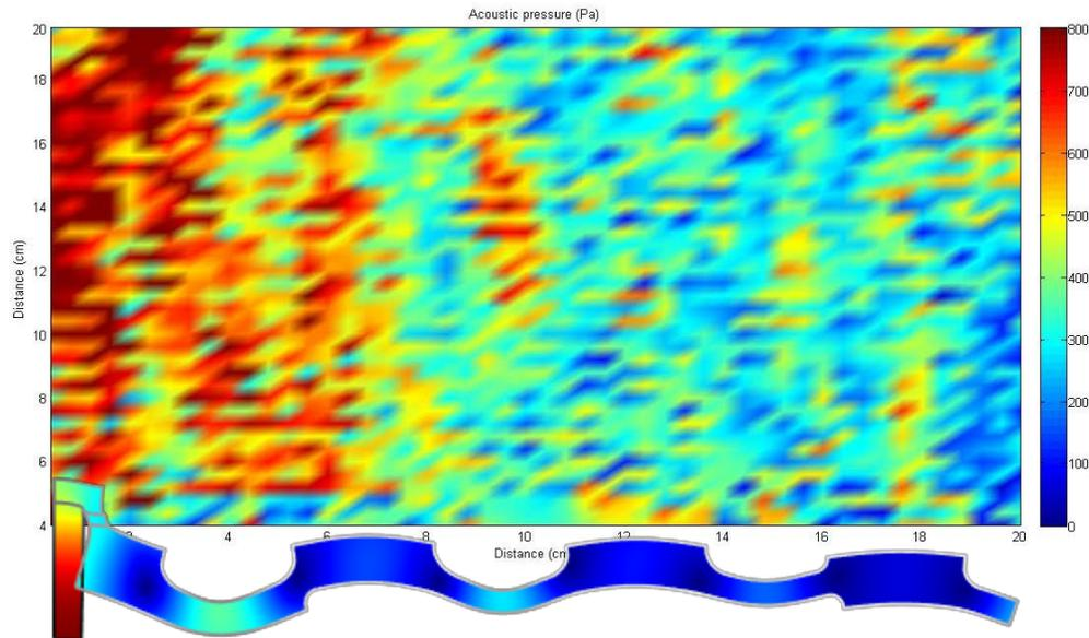
Figure 5: Experimental acoustic field generated by a power ultrasonic transducer with stepped circular plate.
