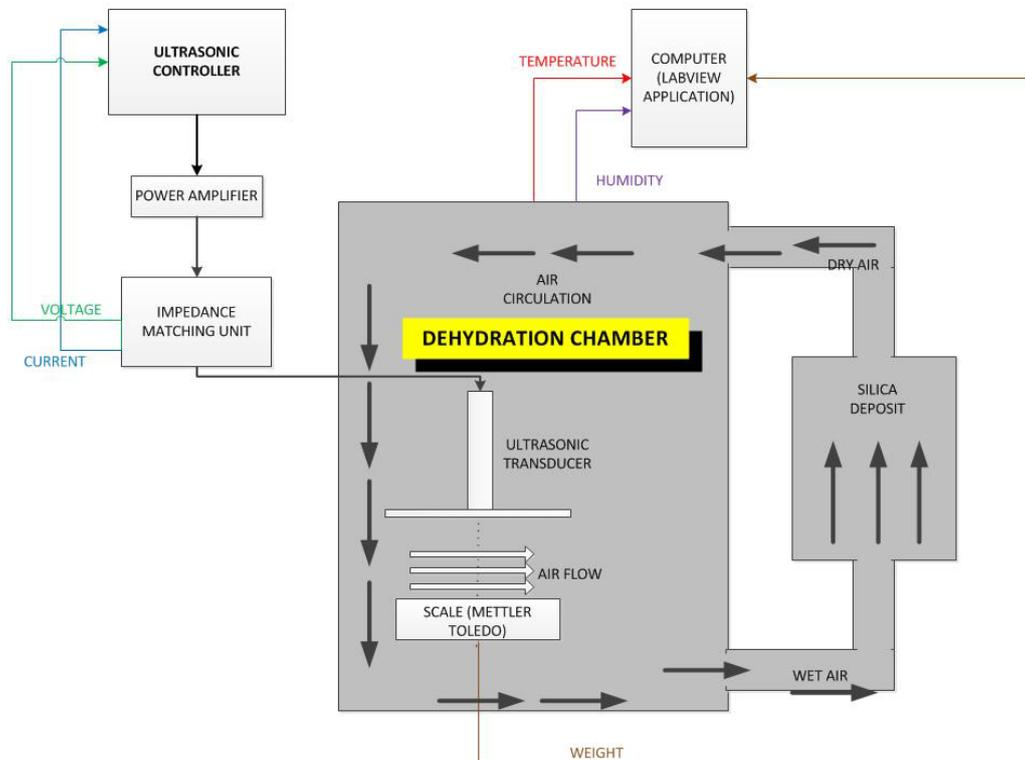
Fig 3. Representation of the dehydration chamber.
