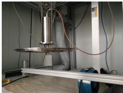
Fig 1. Stepped circular plate transducer in the dehydration chamber.
