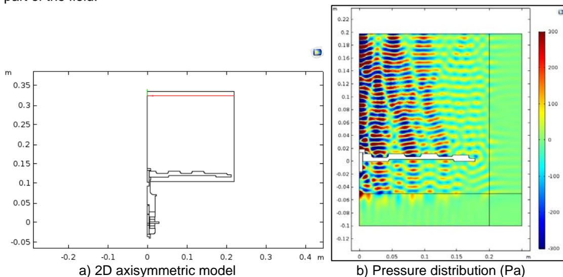
Figure 4: Ultrasonic near field generated by the transducer.
