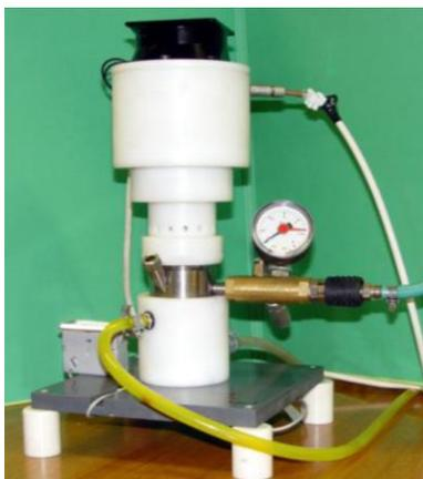
Figure 1. Ultrasound reactor for low-pressure hydrogenation reactions. Reprinted with permission from [2]. Copyright 2013 Elsevier.
