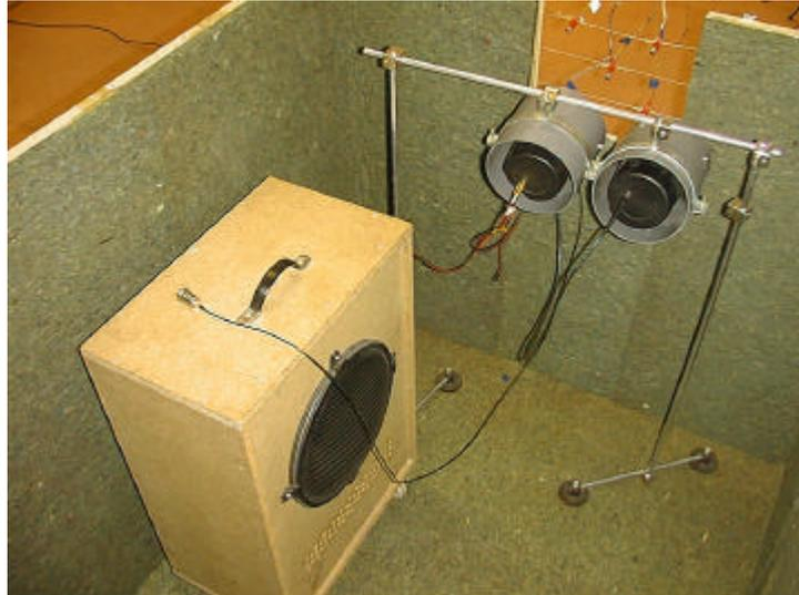
Figure 2. Location of the sound sources and control microphones.
