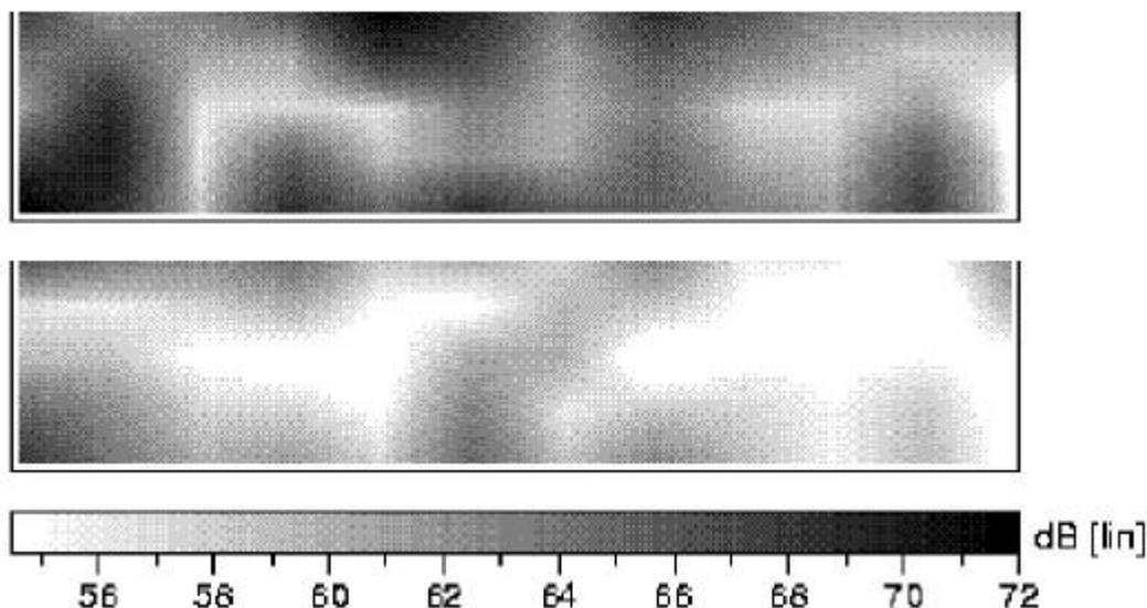
Fig. 5 Spatial distribution of the sound pressure level in the compartment of an ICE high speed coach with (below) and without (above) active control
