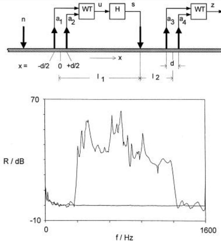
Fig. 4 Principal arrangement and transmission loss of an active reflector
