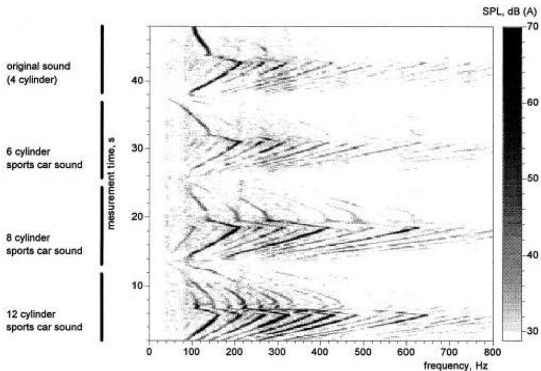
Fig. 6 A weighted sound pressure spectra at the driver's ear for four consecutive run-ups with different engine sounds.
