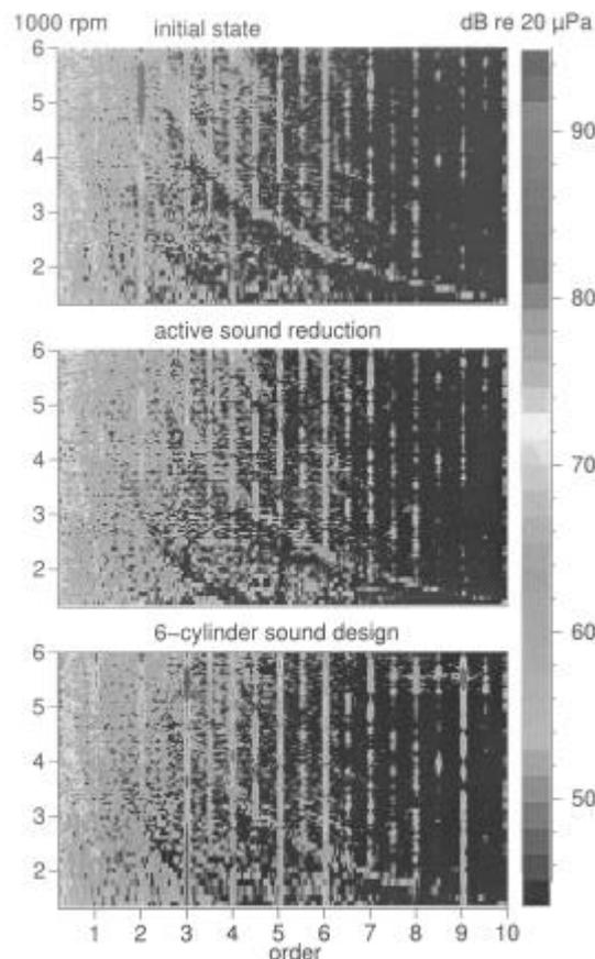
Fig. 7 Order spectra of the sound level at the drivers position during a slow run-up on the road
