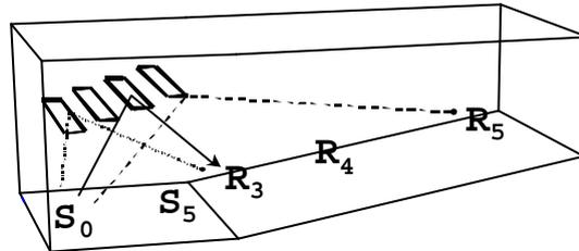
Figure 3. The reflector array. Source S5 is about 1 m from receiver R1 (not shown).
