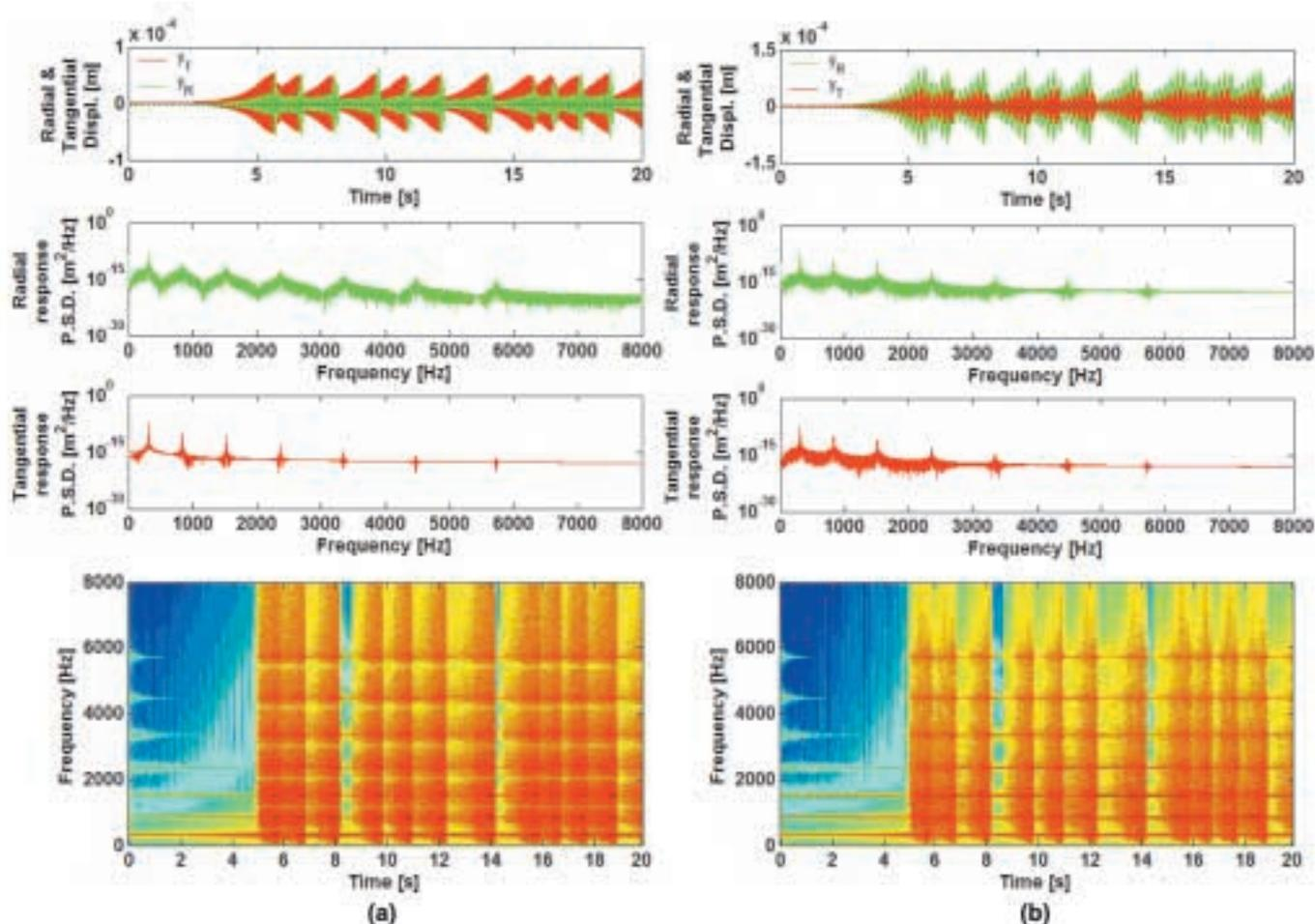
Figure 5 – Time-histories, spectra and spectrograms of the dynamical response of Bowl 2 to friction excitation when  $F_N = 1\text{ N}$ ,  $V_T = 0.5\text{ m/s}$ : (a) at the bowl/*puja* travelling contact point; (b) at a fixed point of the bowl's rim
