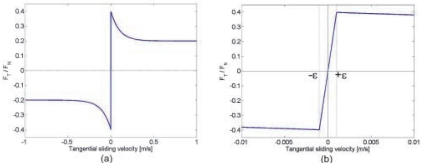
Figure 2 – Evolution of the friction coefficient with the contact relative tangential velocity ( $\mu_\infty = 0.2$ ,  $\mu_s = 0.4$ ,  $C = 10$ ): (a) For  $-1 < \dot{\tilde{y}}_t < 1$ ; (b) For  $-0.01 < \dot{\tilde{y}}_t < 0.01$
