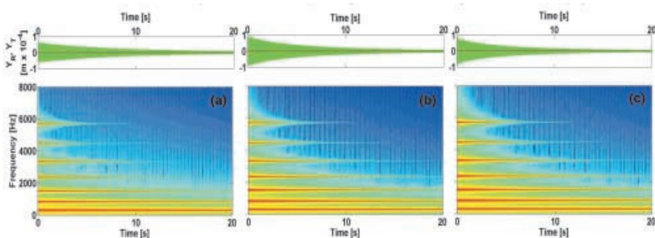
Figure 3 – Displacement time histories (top) and spectrograms (bottom) of the response of Bowl 2 to impact excitation with different values of the bowl/*puja* contact stiffness: (a)  $10^5$  N/m ; (b)  $10^6$  N/m ; (c)  $10^7$  N/m
