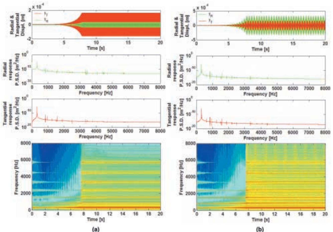
Figure 4 – Time-histories, spectra and spectrograms of the dynamical response of Bowl 2 to friction excitation when  $F_N = 3$  N,  $V_T = 0.3$  m/s: (a) at the bowl/puja travelling contact point; (b) at a fixed point of the bowl’s rim
