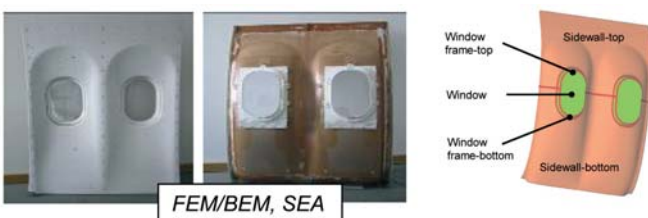
Figure 8.- Side wall panel of an aircraft and its SEA model
